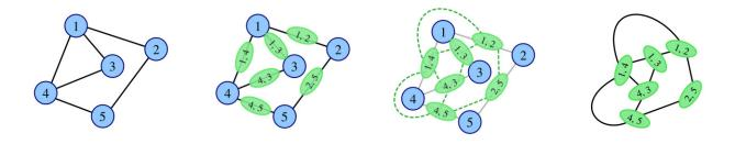
A maximum weighted matching in a simple undirected weighted graph is defined as a set of edges where no two edges share a common vertex and the sum of the weights of the edges in the set is maximized.
